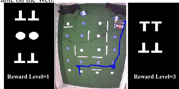
Figure 13. After learning two sequences, the robot selects the most rewarding one performing a decision making process. The learned sequences are depicted on the two sides; the solid line represents the selected trajectory during the testing phase.
