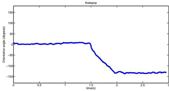
Fig. 6. Heading angle of the agent during a 3s simulation where after a forward movement, a on-the-spot rotation of  $130^\circ$  is performed.
