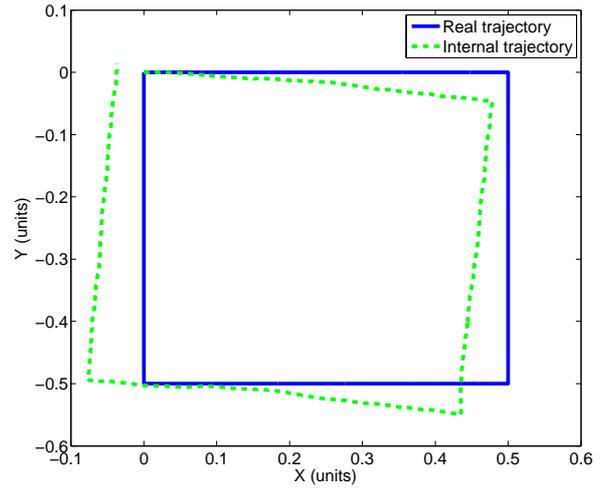
Fig. 9. Comparison between the real trajectory followed by the agent and the estimated position stored in the EB.
