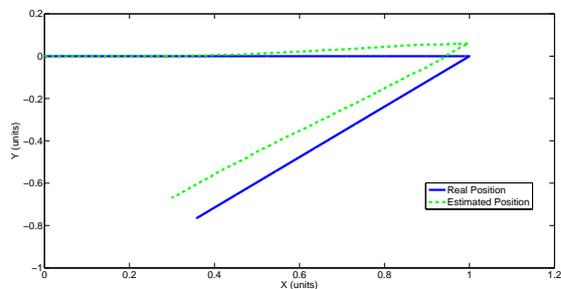
Fig. 8. Comparison between the real trajectory followed by the agent and the internal estimated position stored in the EB.
