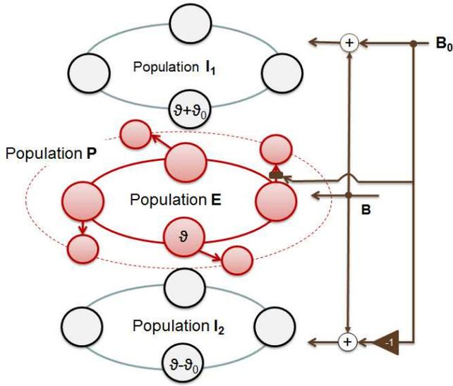
Fig. 4. Four ring network used to model the EB behavior and to reproduce the detour experiments. The external input  $B$  acts as a gate for the population P avoiding an integration during the turning on the spot manoeuvres.
