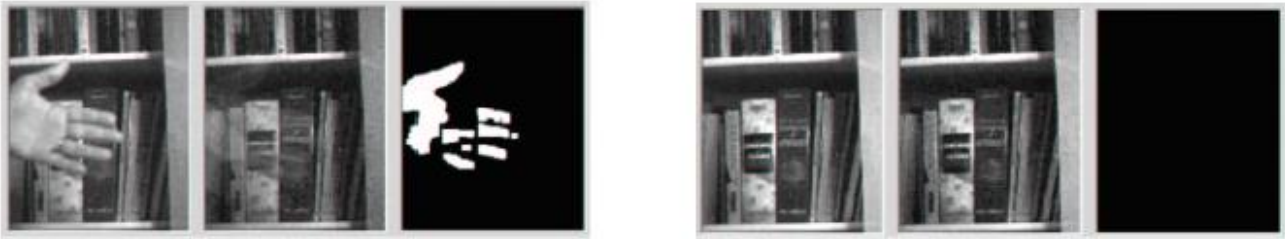
Fig. 6. The left hand side images are the input images, the middle ones are the updated background model, while the right ones are the extracted features. The algorithm cannot extract the object in those places, where the input image is in saturation.
