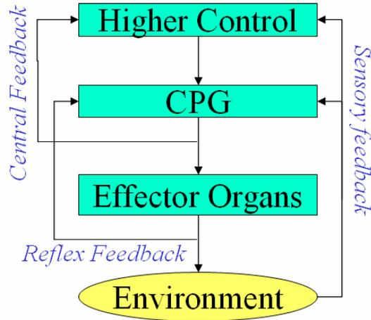
Fig.1 The Central Pattern Generator Scheme
