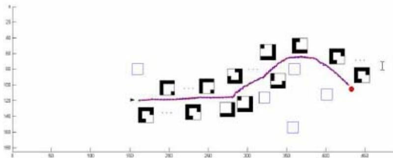
Fig. 11: Navigation through Turing patterns and associated actions in a simulated rover
