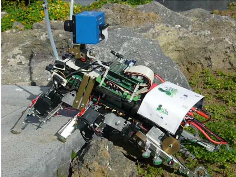
Fig.13: Gregor III: a cockroach inspired robot used as test-bed for the designed cognitive architecture within the SPARK project.
