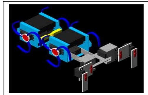
Fig.3: Mechanical model of the Trinacry\_bot robot.
