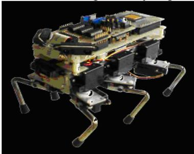
Fig.1: The MiniHex robot. The low level locomotion control is based on the CPG paradigm.
