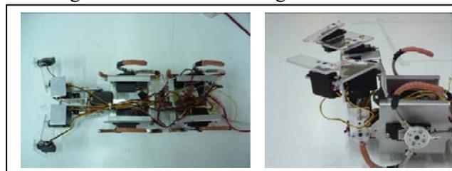
Fig.4: Different configurations of the Trinacry\_bot. (a) The frontal legs are used to climb obstacles. (b) Legs are used as manipulator to take objects.
